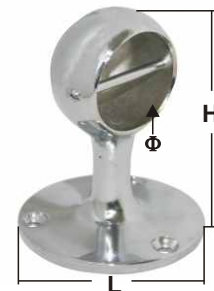
END STANCHIONS Casted AISI 316 With thread pin ITEM NO. \Phi L H Weight/g 009646 36 70 86 293
