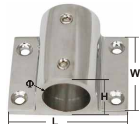
TUBE HOLDER casted AISI 316 ITEM NO. For tube \Phi L mm W mm H mm Weight B19-019 22 mm 58 46 29 160g B19-020 25 mm 61.5 46 33 180g
