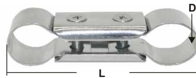
GRAB HANDLE CONNECTION stamped AISI 316 ITEM NO. L mm D mm Weight/g 009656 90(3-1/2") 22(7/8") 009664 90(3-1/2") 25(1")
