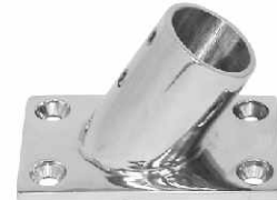
60° RECTANGULAR BASE casted AISI 316 ITEM NO. Tube O.D. Base mm Weight/g 009617 32mm(1-1/4") 82x42 250
