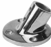
60° ROUND BASE casted AISI 316 ITEM NO. Tube O.D. Base Weight/g 009612 32mm(1-1/4") 75mm 260
