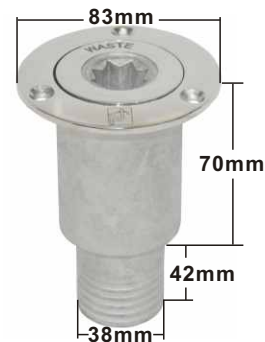
WASTE according ISO8099:200 AISI 316 ITEM NO. Weight B16-002 760g
