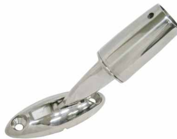
FIXING PLATE WITH QUICK RELEASE casted AISI 316 Disengage turning the central part. ITEM NO. Base mm Tube O.D. Weight/g 009640 89x32 22mm(7/8") 320 009641 89x32 25mm(1") 250 009642 89x32 30mm(1-3/16") 300
